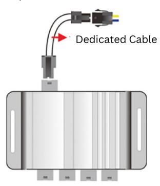
Please use the dedicated connection line provided by the dealer to connect to the data interface of the terminal, and the terminal will automatically recognize the temperature box when it is turned on.
